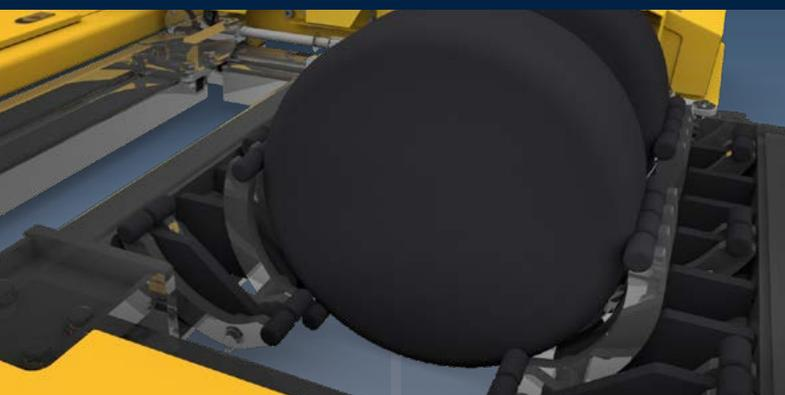
Depending on the size of the nose wheel, the 28 individually movable nose wheel clamps are gently pressed against the nose wheel to hold it securely.
