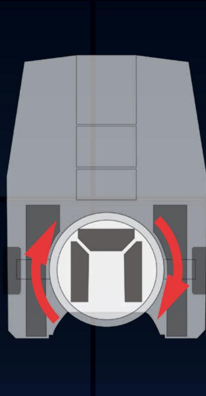
The nose landing gear is clamped on a rotating turntable to prevent damage to the nose wheel if the maximum turning angle of the nose wheel is reached. The aircraft tractor can continue to turn, but the turntable remains stationary.
