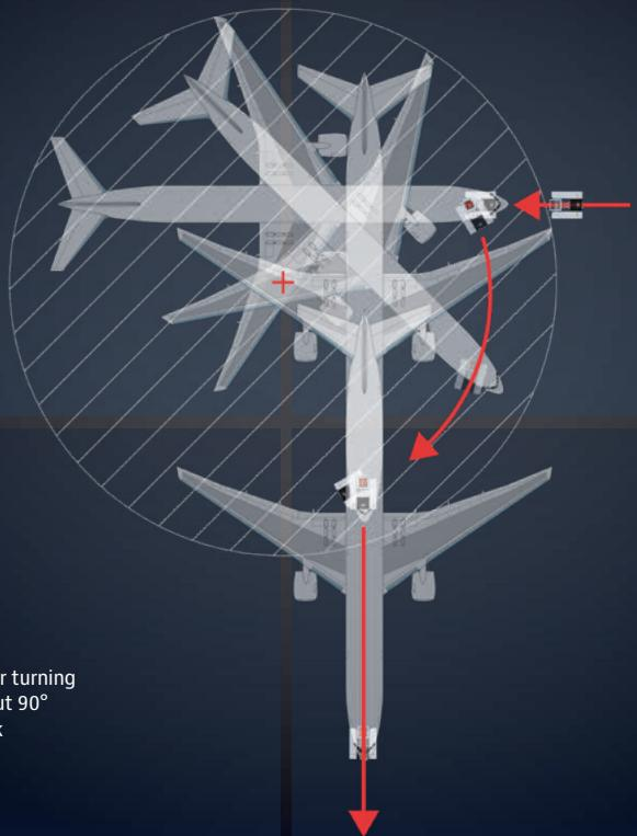
Manoeuvring with Mototok is the easiest and safest by far. With Mototok, both turning the nose gear and moving the aircraft are two completely different movements. The fuselage and wingtips remain in position whilst turning the nose gear. The result is a minimum requirement of space. This example shows that turning an aircraft by 90° reduces manoeuvring space to a circle.
