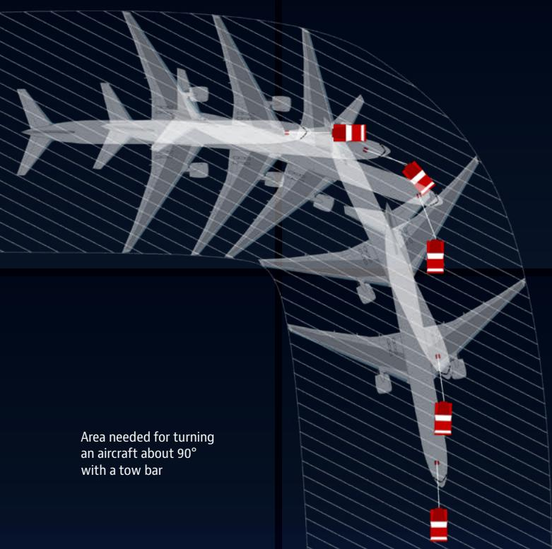
Area needed for turning an aircraft about 90° with a tow bar
