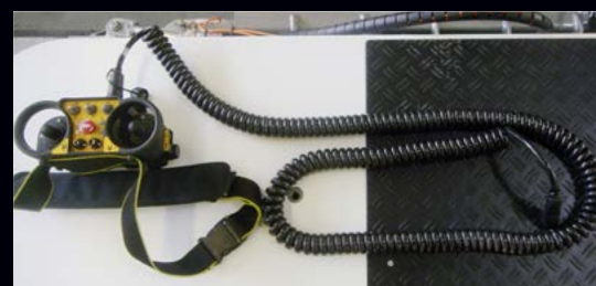
Cable for Remote Control Insert the optional coiled cable connection to switch off the radio function automatically.
