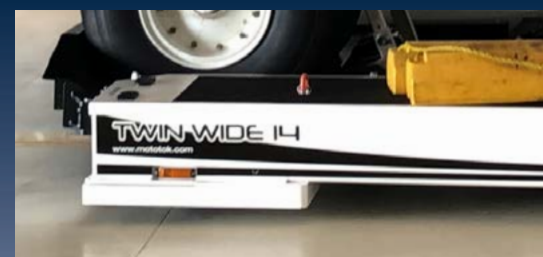
Additional weight For more grip on slippery surface
