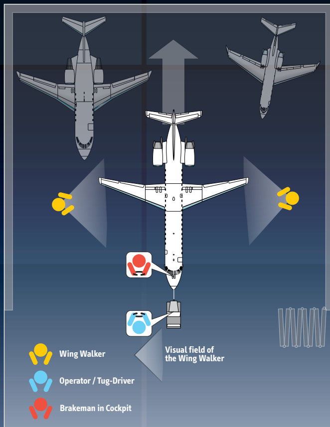
Towing with a conventional Tractor: At least 4 Persons needed
