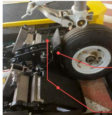
Cage with integrated torque measuring equipment (single wheel)
