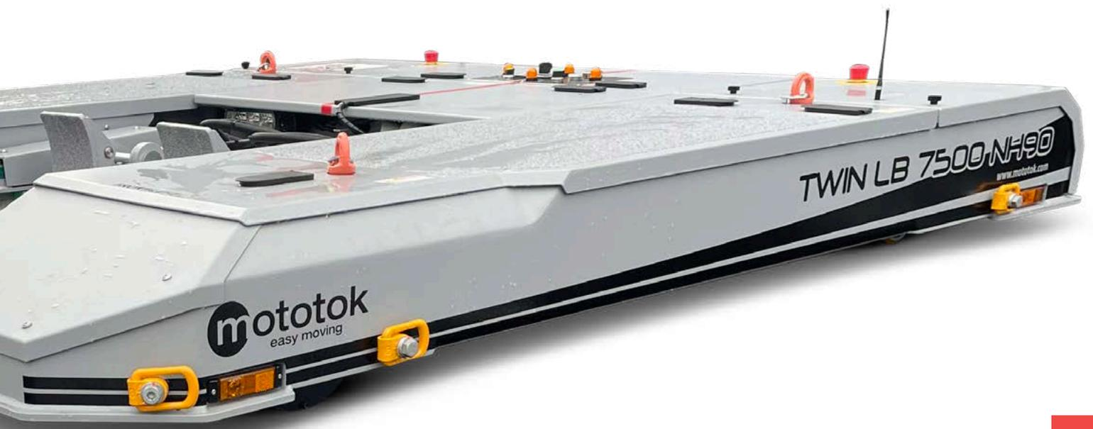
Loading and unloading the nose gear is triggered by pushing a button on the remote control. Of course, the loading or unloading sequence can also be carried out manually.
